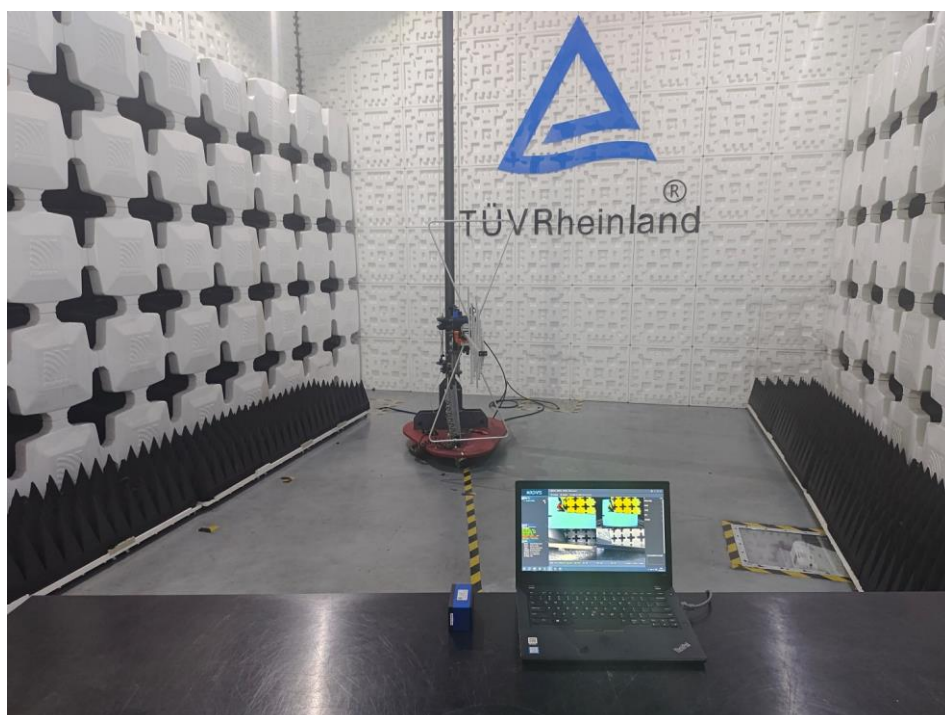
Photograph 2: Set-up for Radiated Emission Below 1GHz
